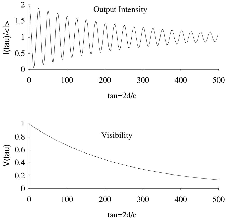
Figure 5-1. Representative plots of output intensity and visibility for a Lorentzian spectral line.
