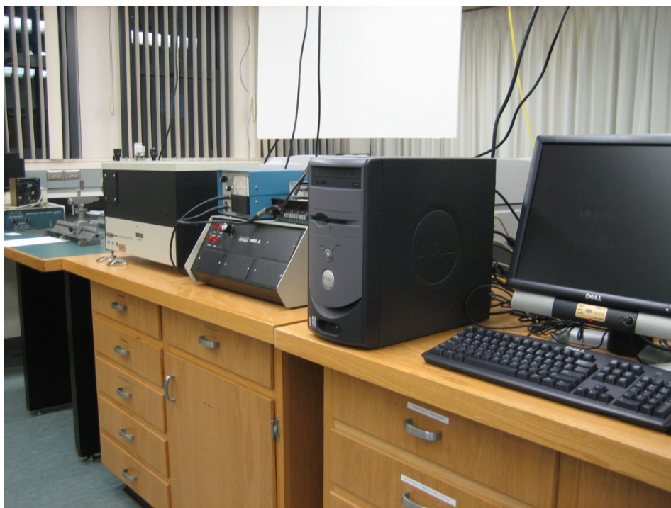
Figure 2.3: The SPEX 500M grating spectrometer with controlling electronics and computer.
